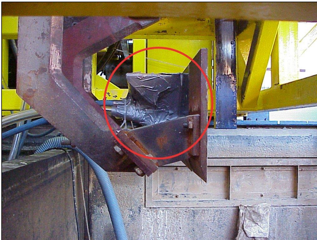
Figure 11-32: Cover with camera behind the blade.
