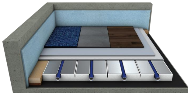
Lightweight floor heating system (Jupiter, 2017)
