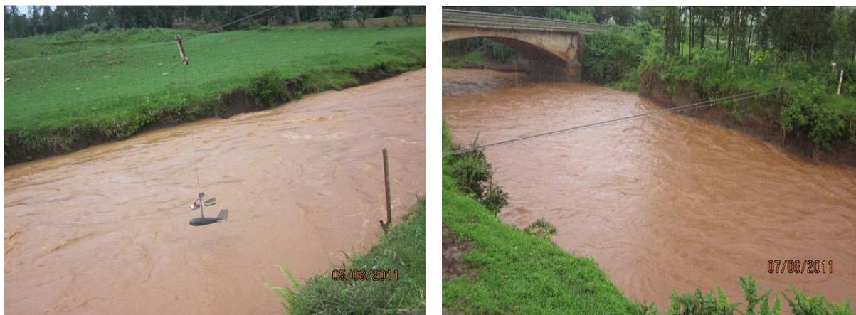
Figure 7.1: Velocity measurements for development of rating curves in Chemoga left and Jedeb rivers right during high flow period (Photo taken by the author August 2011).
