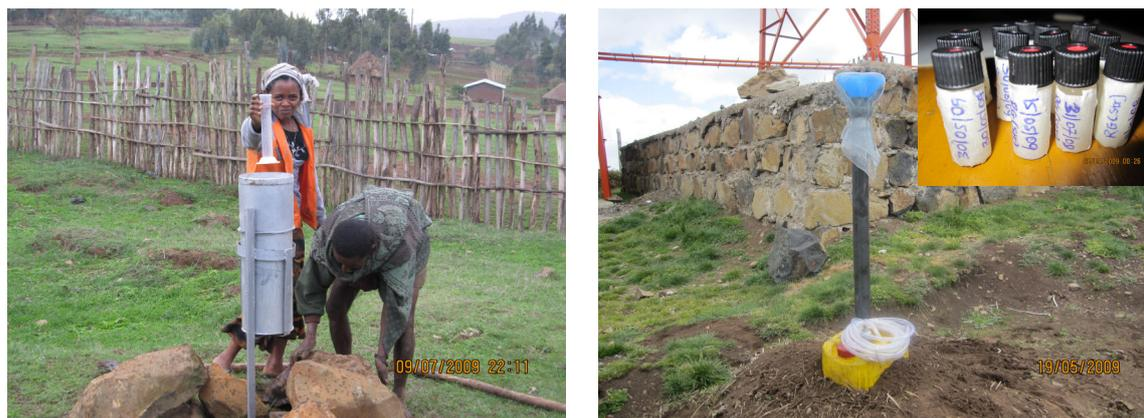
Figure 6.2: Sample manual rain gauge (left) and Precipitation water samples collector for isotope analysis (right). The inset figure right is the 2 mL sampling bottles for the different water samples (precipitation, springs, and river).
