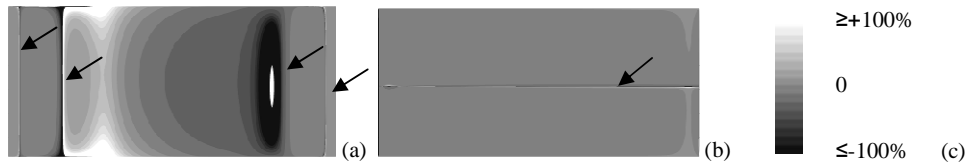
Figure 13. Comparison of unwrapped phase maps from camera 1 for the cylinder sample with x shear (a) and y shear (b). (c) scale where each grey level represents a range of 12,5% of difference.
