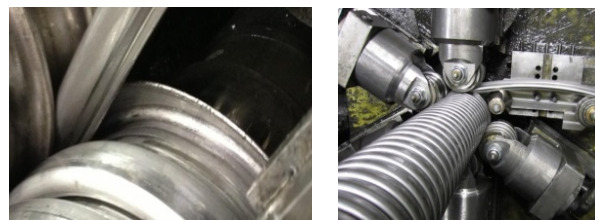
Figure 6. Manufacture process of carcass layer [41]
