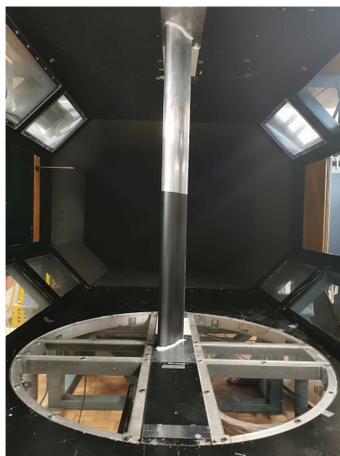
FIGURE 1 | Side view of the test section with the mounted airfoil (left) and the nondimensionalized geometry of airfoil DU91-W2-150 with locations of pressure taps marked with circles (right).
