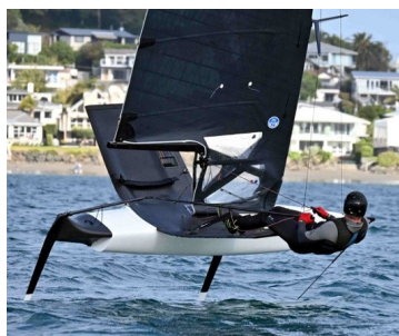
(a) Bieker Moth sailing in foiling mode at upwind point of sail
