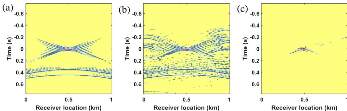
**Figure 2** (a) Focused shot gather from the coarse aliasing data in Figure 1a. (b) Focused shot gather from the blended data in Figure 1b. (c) Focused shot gather after 400 spgII iterations using sparse inversion.
