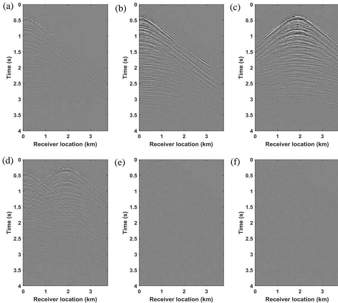
**Figure 3** Unblended, coarse shot gather (a) and blended shot gather (d). Deblended and reconstructed left shot gather (b) and right shot gather (c) after 800 spg11 iterations ( $Q=12.46$  dB). (e), (f) are the differences between Figure 3b, Figure 3c and the corresponding coarse input data at the known traces.
