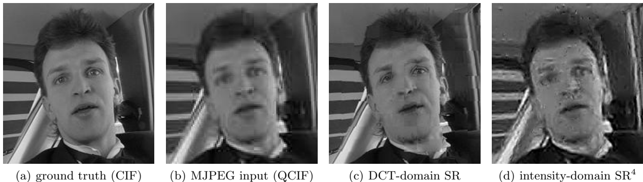
Figure 7. Comparison of two-time SR synthesis of an MJPEG compressed frame in the DCT and intensity domain.
