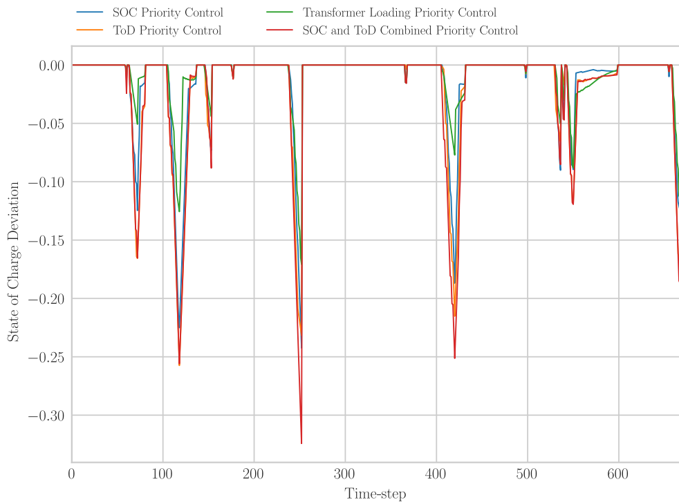
Figure 4.12: This plot shows the difference in SOC between all charging strategies compared to the uncontrolled strategy in the RVO scenario. Compared to the Base scenario, the higher charging powers in this scenario have increased the SOC deviation during short charging periods and further decreased the SOC deviation during the long charging periods.
