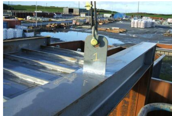
Figure 1.0.2 A welded lifting lug (AUTODESK.COMMUNITY [3] )
