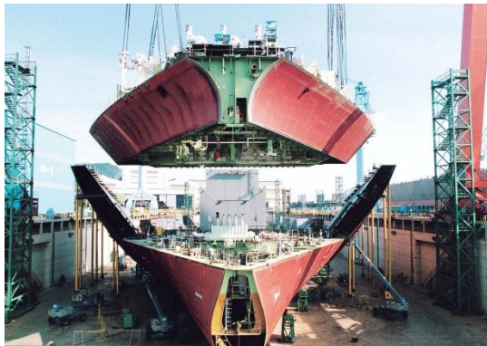
Figure 1.0.1 A lifted section in building process (World maritime news [2] )
