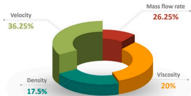
Fig. 20. Extent of influence of different factors on the MSS gas quenching process.
