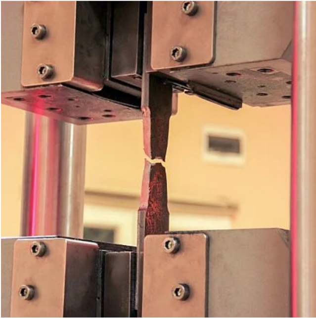
Figure 4. Destructive Testing - Tensile Test, Source: MFE Inspection Solutions (2024)
