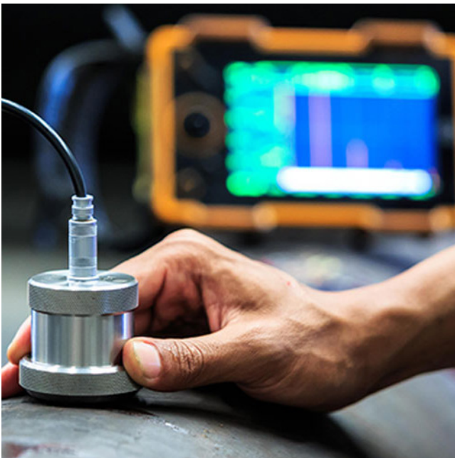
Figure 5. Non-Destructive Testing - Ultrasonic Testing, Source: Format NDT (n.d.)
