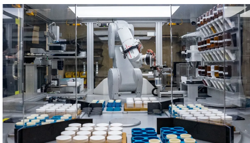
Figure 1.1: The A-Lab at University of California, Berkeley. Guided by a learning algorithm, and as part of a broader experimentation process, this robot arm can grab, open, and dispense materials within its reach. This creates a streamlined process for precise and reliable powder dosing. Photo credit: Marilyn Sargent/Berkeley Lab (licensed under CC BY 4.0 via Springer Nature).
