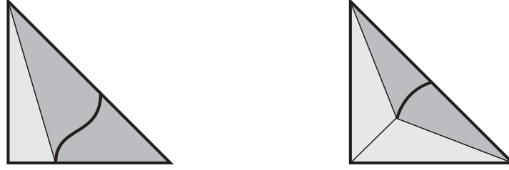
Figure 2.3: Examples of subtriangulation of elements crossed by NURBS-based discontinuities into integration elements: on the left, an internal discontinuity element is illustrated, while the right image represents the case of an element containing a crack tip. The darker color indicates the integration elements sharing a NURBS edge, that will need an ad hoc construction for the enrichment functions.
