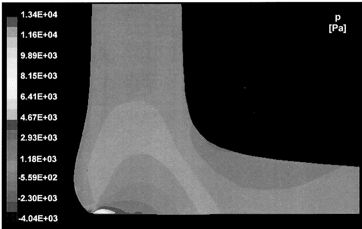
Figure 7.17: Contours of pressure in the heel region (coarse mesh,  $n = 4$ ).
