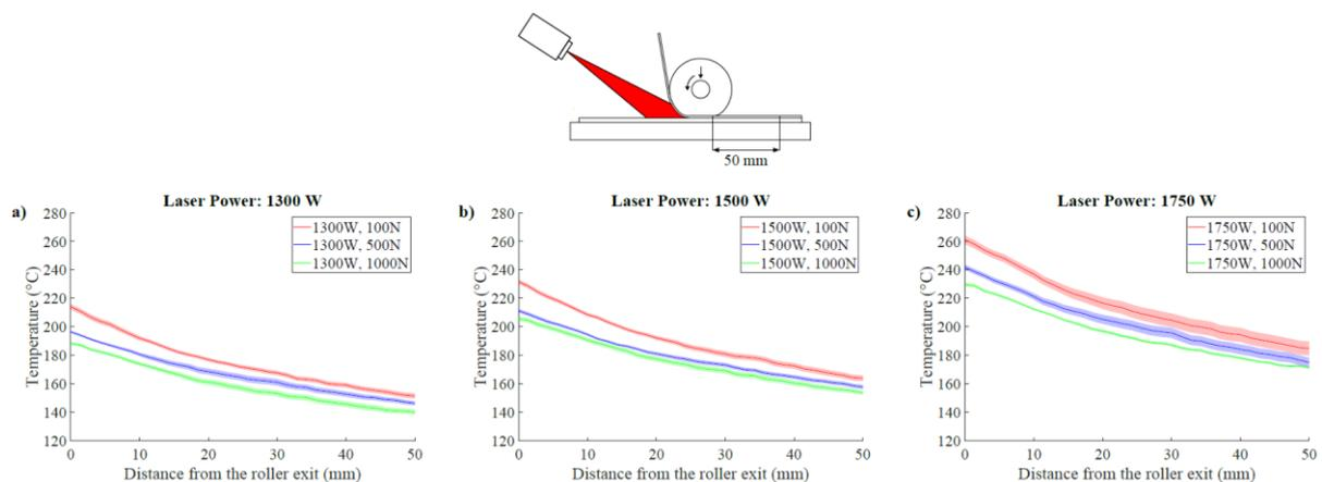
**Figure 7. Average tape temperatures at the roller exit on the top surface of the fifth tow for different compaction forces and laser powers**
