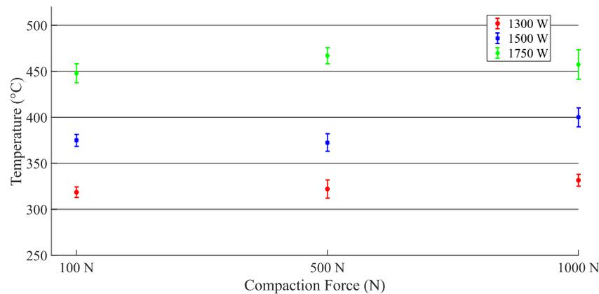
**Figure 6. Average tape inlet temperatures for the fifth tow at each laser power and compaction force.**
