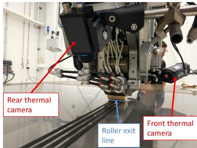
**Figure 2. Front and rear thermal cameras on the fiber placement machine to measure the tape inlet and exit temperatures during the process.**
