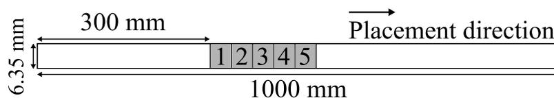
**Figure 4. Extraction locations of five samples for intimate contact investigation.**
