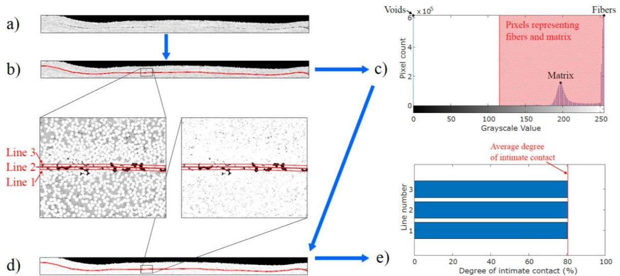
**Figure 5. Methodology for intimate contact measurement at the topmost interface from cross-sectional images.**
