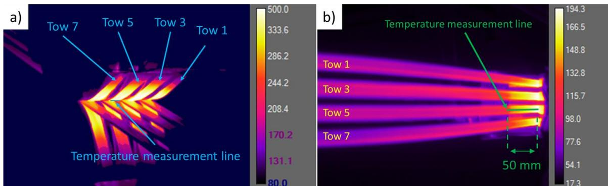
**Figure 3. Thermal images and measurement lines from: a) the front thermal camera b) the rear thermal camera**
