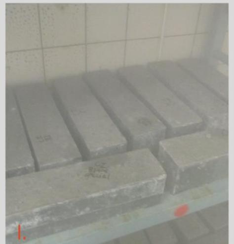
Half of the concrete mixture was then poured in the pre-oiled moulds (Fig. 4.3g and h), that were positioned on the vibrating table. During the first casting day, oil was used, but the second and third casting Vaseline was applied, because it proved to be much easier during un moulding.
