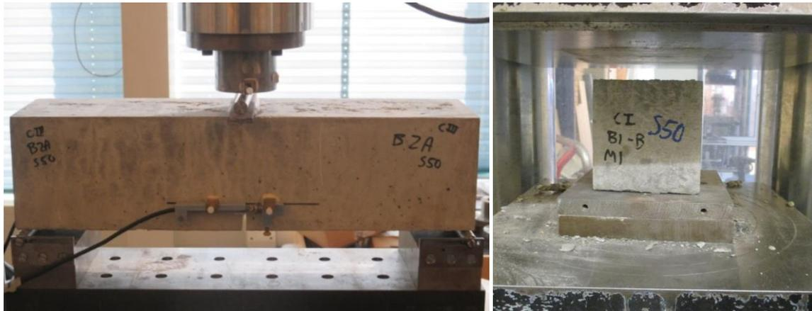
Fig. 4.6: Left: three-point bending test setup. Right: Compressive strength test set-up.
