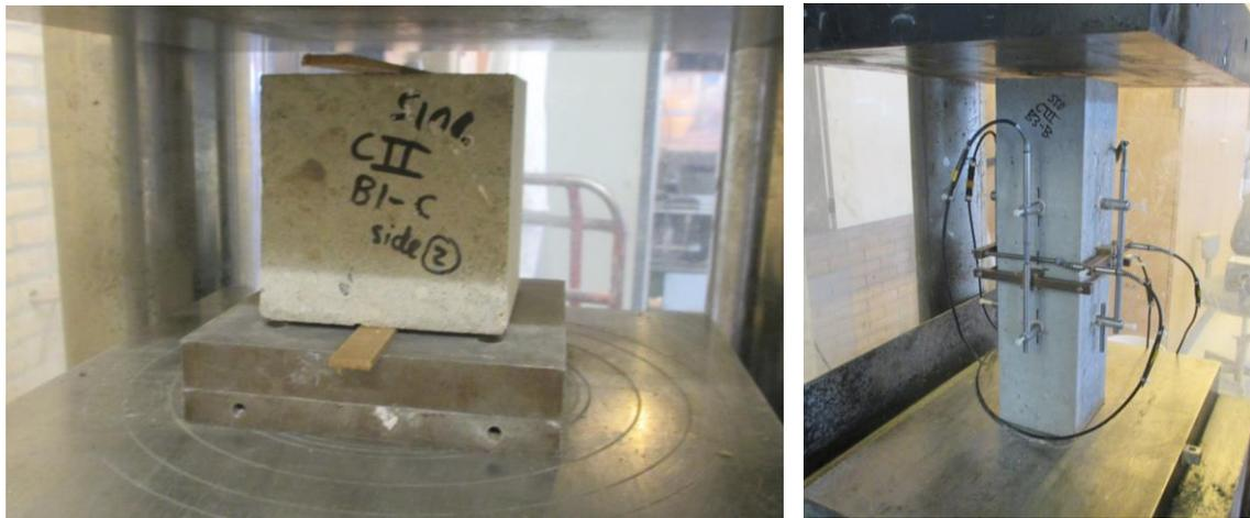
Fig. 4.8: Left: Splitting tensile strength test set-up. Right: Elastic modulus test set-up.
