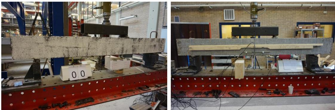
Fig. 4.10: Test set-up. Left: painted side of beam for image analysis. Right: LVDTs to measure deformation.
