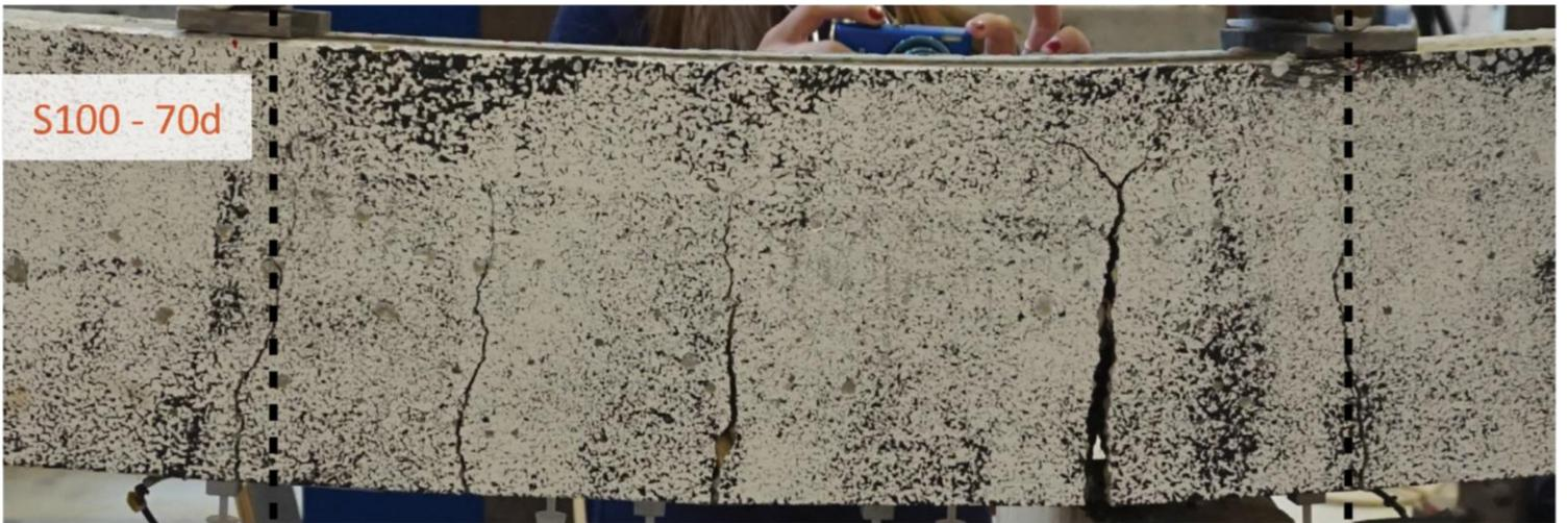
Fig. 5.11: Crack patterns in alkali-activated beams, after failure. Dotted lines indicate the constant moment zone.
