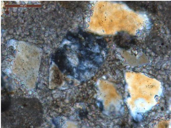
(c) S11. Corroded quartz grain with calcite crystals on the left. Polycrystalline quartz in the middle.
