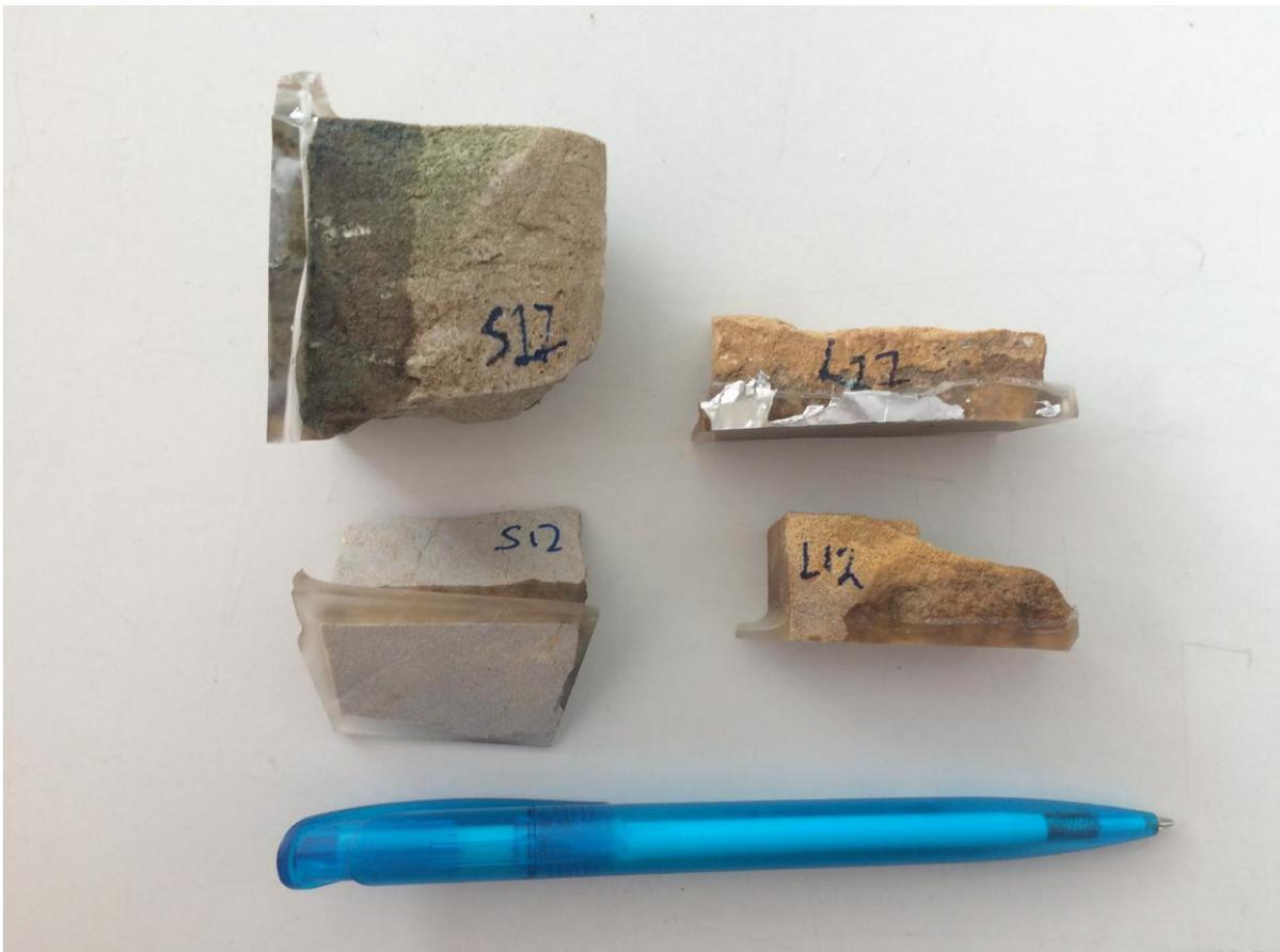
Figure 5.1: The four impregnated samples from which the sections were created
