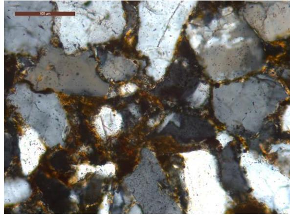
(b) L12. Quartz grains with ferroan cement in between.
