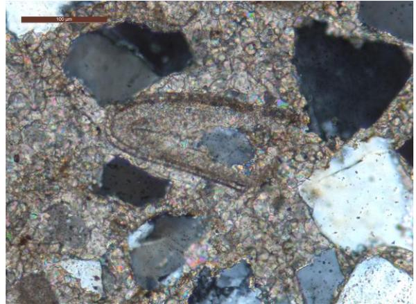
(b) S12. Micritised fossil filled up with cement and quartz grain.
