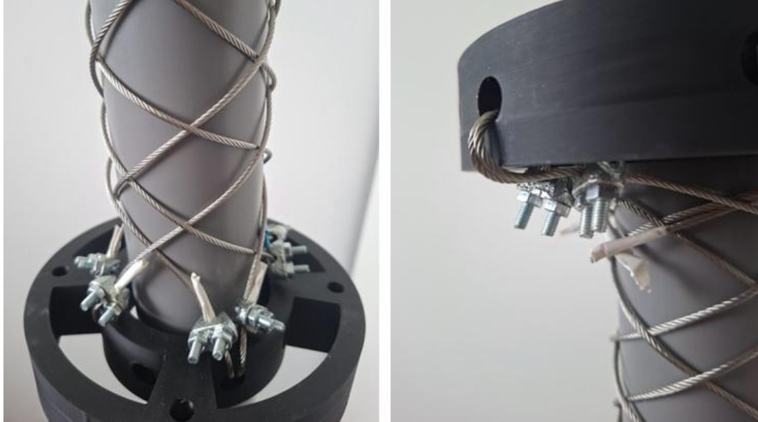
Figure 5.2: Steel wire braid fabricated using the same method, with U-bolt clamps fixing the wire ends
