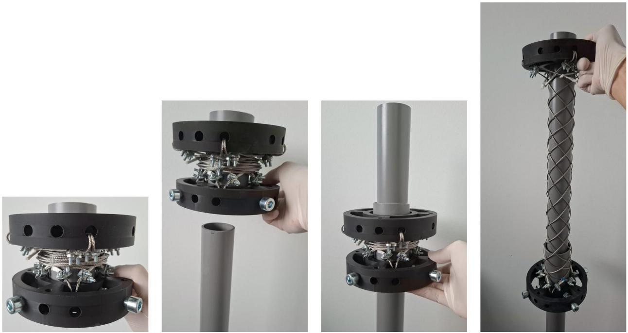
Figure 7.4: Anti-bunching support sleeve concept for controlled deployment, shown on the steel wire prototype
