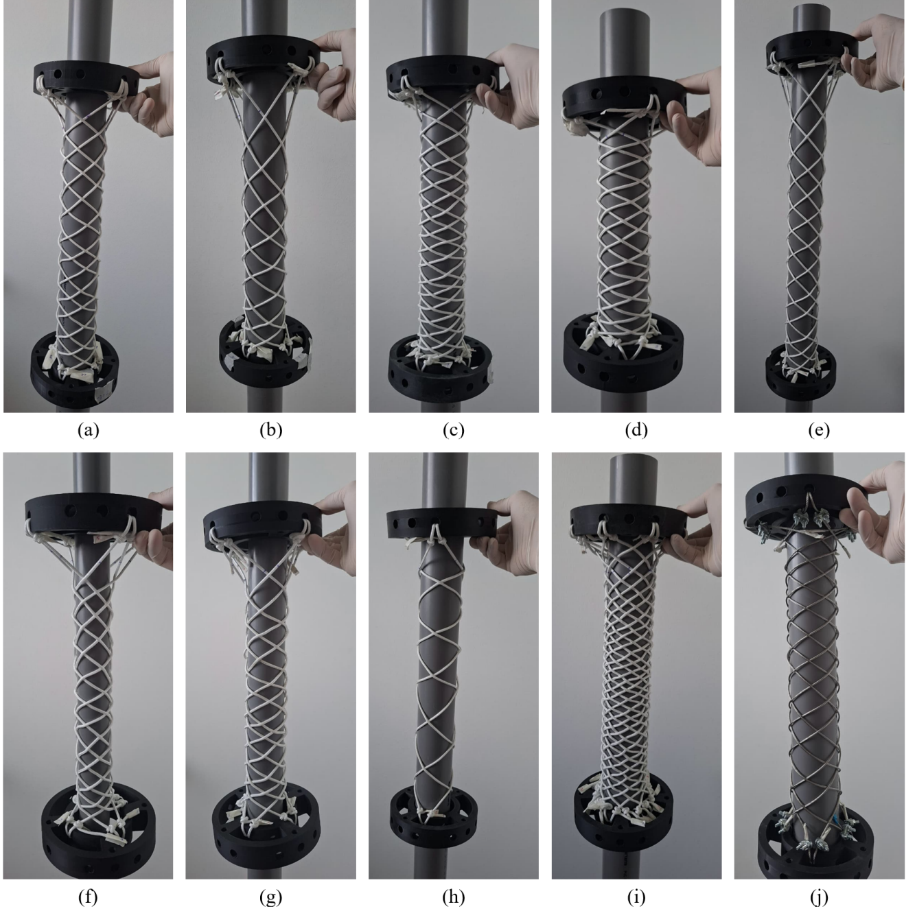
Fig. 6. Fabricated configurations of the test matrix. (a) Baseline. (b) N = 2 . (c) N = 4 . (d) H = 200 mm. (e) H = 600 mm. (f) r_c = 20 mm. (g) r_c = 25 mm. (h) n = 2 . (i) n = 8 . (j) Steel wire.
