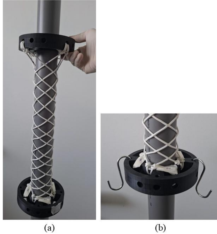
Figure 5.3: Baseline configuration and ring weight variation. (a) Baseline: N=3 , H=400 mm, r_c=30 mm, n=4 , W_{\text{ring}}=0.98 N, polyamide rope. (b) Hooks attached to the bottom ring for additional mass
