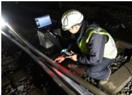
(a) Measurement using HandyScan
