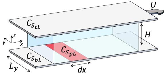
Figure 1: Sketch of the system under study, composed of two solid plates separated by a distance  $H$  with the top plate sliding at a speed  $U$  relative to the bottom plate. The case of a chemical heterogeneity in the bottom plate is also illustrated
