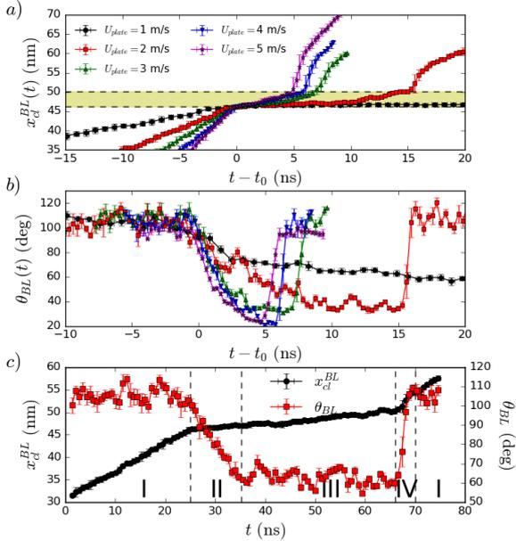
Figure 4: a) Evolution of the receding contact line location on the bottom plate (BL) for  $C_{SpL} = 1.0$  and different plate velocities  $U$ . b) Evolution of the receding contact angle on the bottom plate  $\theta_{BL}(t)$  for  $C_{SpL} = 1.0$  and the same velocities as in subplot a). c) Evolution of the contact line location and the contact angle for the BL contact line for  $C_{SpL} = 0.9$  and  $U = 1$  m/s. The different regions are delimited by vertical dashed lines.
