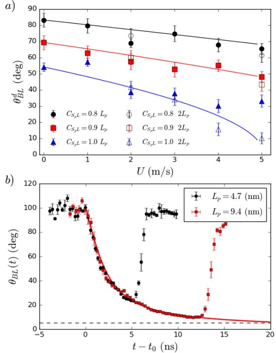
Figure 7: a) Contact angle of the BL contact line in region III before escape from the patch for the different simulations performed. The full and open symbols correspond to the smaller and the larger  $L_p$ , respectively. The lines corresponds with the results from Eq. 14. b) Evolution of  $\theta_{BL}(t)$  for  $C_{S_p L} = 1.0$ ,  $U = 5$  m/s and both patch lengths  $L_p$ . The continuous line corresponds with the results from Eq. 11.
