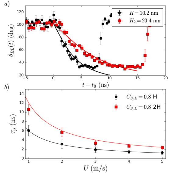
Figure 6: a) Evolution of  $\theta_{BL}(t)$  for  $C_{SpL} = 1.0$  and  $U = 3$  m/s for both plate separations. The lines correspond to the estimation from Eq. 11. b) Pinning time versus plate velocity for  $C_{SpL} = 0.8$  and both plate separations. The lines corresponds to the predictions from Eq. 12.
