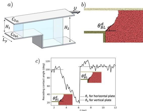
Figure 8: a) Scheme of the physical heterogeneity. b) Snapshot of a simulation with the receding contact line pinned at the physical heterogeneity. c) Evolution of the contact angle on the edge. The lines at the left and the right side represent respectively the receding contact angle for the horizontal plate and the equilibrium contact angle for the vertical edge.
