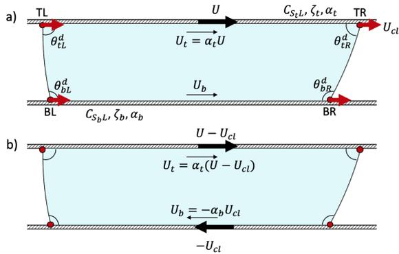
Figure 2: a) Framework of reference 1 where the top plate moves at constant velocity  $U$  and the bottom plate remains at rest. Here, the four contact lines move at constant velocity  $U_{cl}$ . b) Framework of reference 2 where the four contact lines remain at rest and the top and bottom plates move at constant velocity of  $U - U_{cl}$  and  $-U_{cl}$ , respectively.
