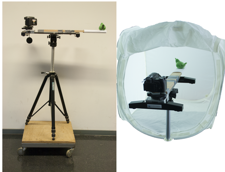
Figure 3.1: The setup for the photography of the object under different lighting conditions. Left: The object and the camera were fixed onto a frame attached to a tripod and placed on a small trolley. This setup could be rolled into the three canonical lighting setups of which one is shown on the right. The ambient lighting scene was created using a white photo tent – which was almost closed during the photography.
