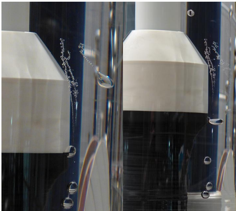
Figure 114: Close-up of dispersion faced (left); Halt of dispersion after water droplet leaves area of high stress (right)
