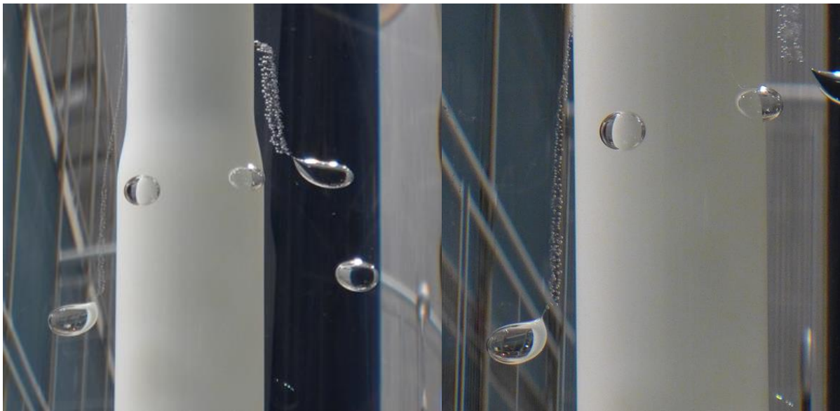
Figure 115: Degradation occurring at top (left); Clear evidence of larger radius resulting in smaller critical field strength (right)
