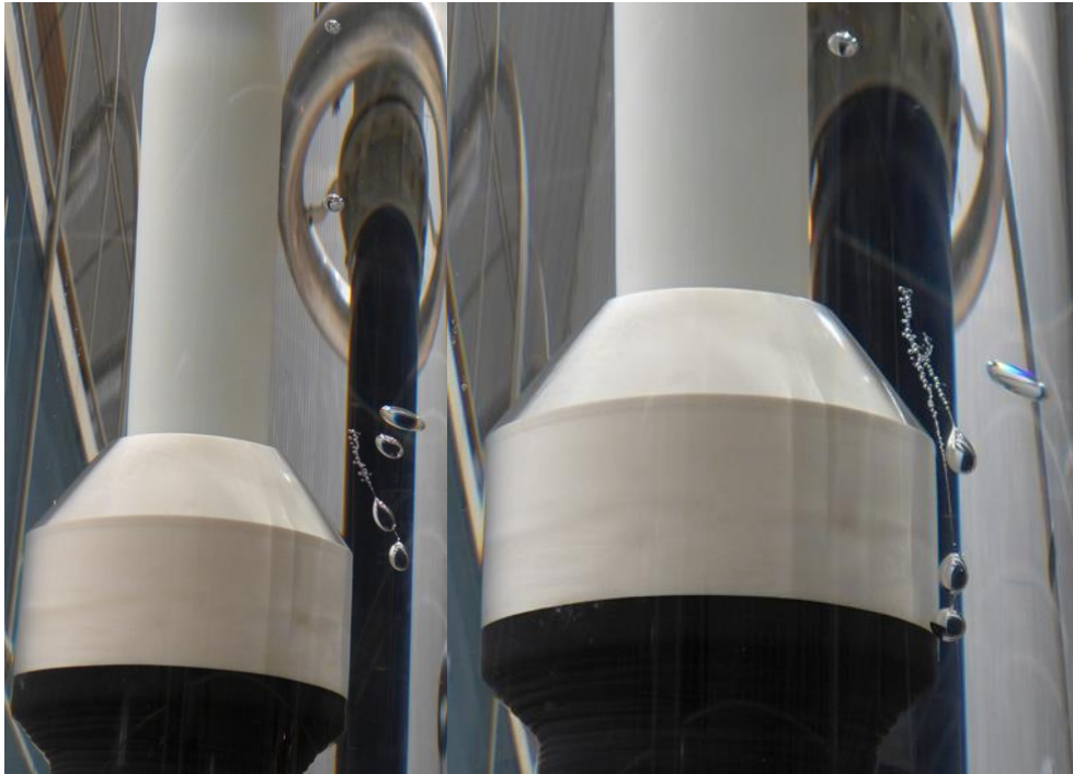
Figure 113: Elongation and dispersion observed (left), Degradation on an elongated water droplet whilst getting dragged down by gravity (right)
