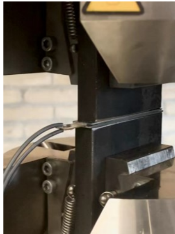
(a) Clamp the piezoelectric plate.
