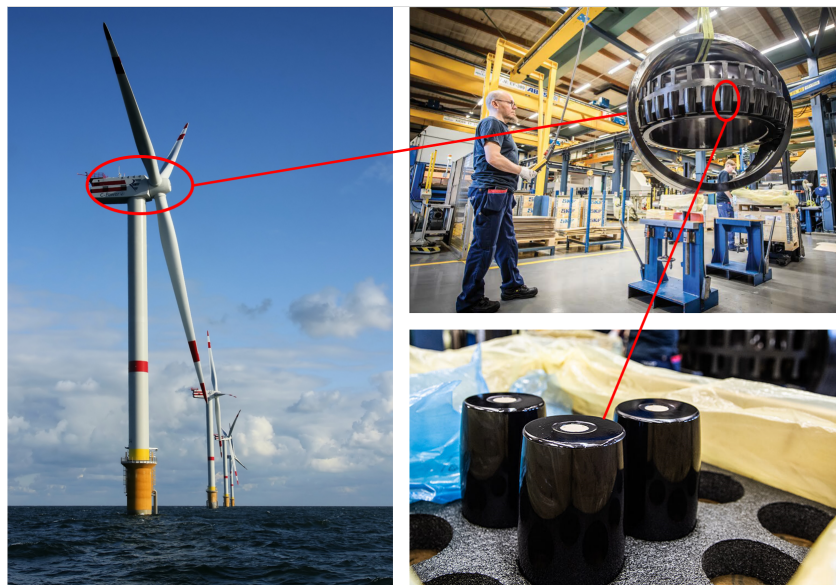
Figure 1.3: Wind turbine bearing with the Sensor Roller.[11]
