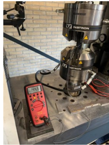
(b) Connect piezoelectric with a multimeter.
