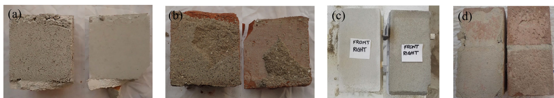
Fig. 13. Top view from the debonded surface of CS and clay masonry specimens: (a-b) cores; (c-d) triplets.
