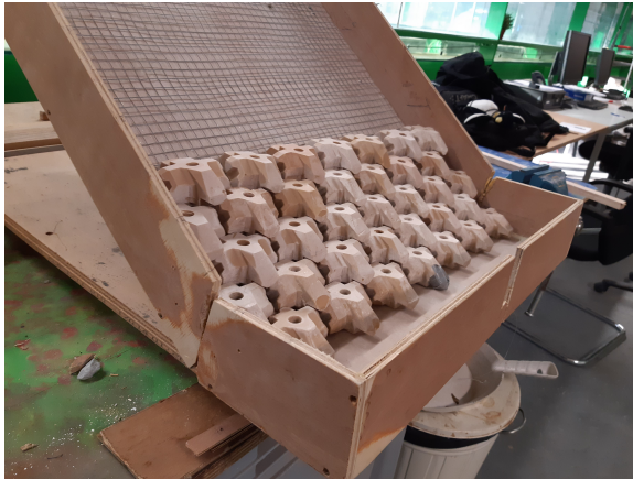
Figure 4.1: The pull-out test set up
