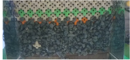
Figure 8.5: Damage of the toe berm at H/D_n * \Delta = 4.8 , \Delta x/D_n = 0.10
