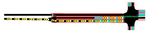
Figure 5.5: Case where spillback is detected, communicated, and processed by TFE (penalty X1000)
