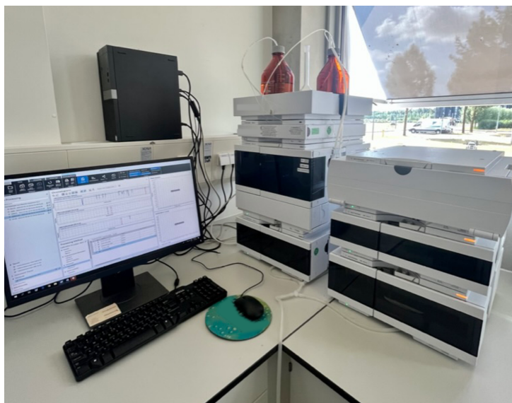
Figure 5.A.14: Agilent Technologies 1260 Infinity II HPLC setup.
