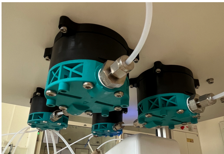
Figure 5.A.8: Pressure dampeners, screwed to the bottom of the BPR-setup.
