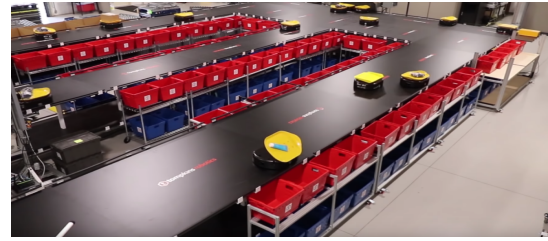
(b) Tompkins Robotics: t-Sort sortation on a tabletop design with tilt tray AGVs [84]
