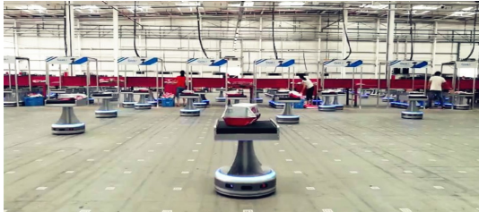
(c) Geek+ S20-warehouse AGV, belt conveyor AGVs [85]
