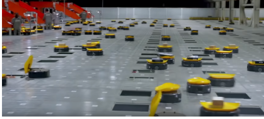
(a) 1.3 \text{ km}^2 sortation transit, chutes beneath every opening in the ground and tilt tray AGVs [83]
