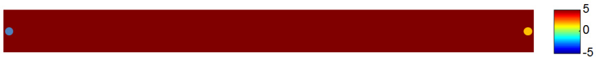
Figure 4.2: Permeability field of the starting model. Permeability values are expressed as the natural logarithm of permeability in mD. The blue and orange dots indicate the injector and the producer respectively.
