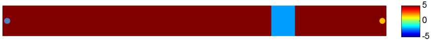
Figure 4.1: Permeability field of a one-dimensional homogenous reservoir model with a low-permeable barrier. Permeability values are expressed as the natural logarithm of permeability in mD. The blue and orange dots indicate the injector and the producer respectively.
