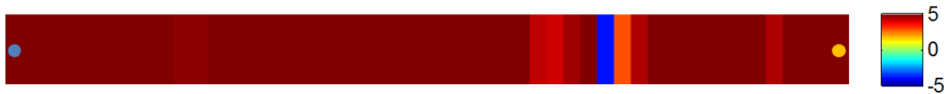
Figure 4.5: Updated permeability field of the 1D reservoir model for experiment #3. Permeability values are expressed as the natural logarithm of permeability in mD.
