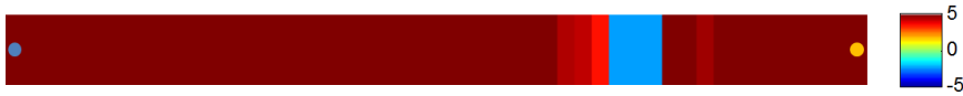
Figure 4.3: Updated permeability field of the 1D reservoir model for experiment #1. Permeability values are expressed as the natural logarithm of permeability in mD.
