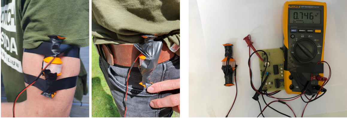
(a) Harvester mounted on the upper arm. (b) Harvester mounted on the waist. (c) Measurement setup for determining delivered power.
