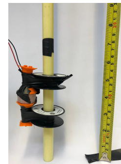
(b) Harvester, sliding along tube, ruler for dimensions.
