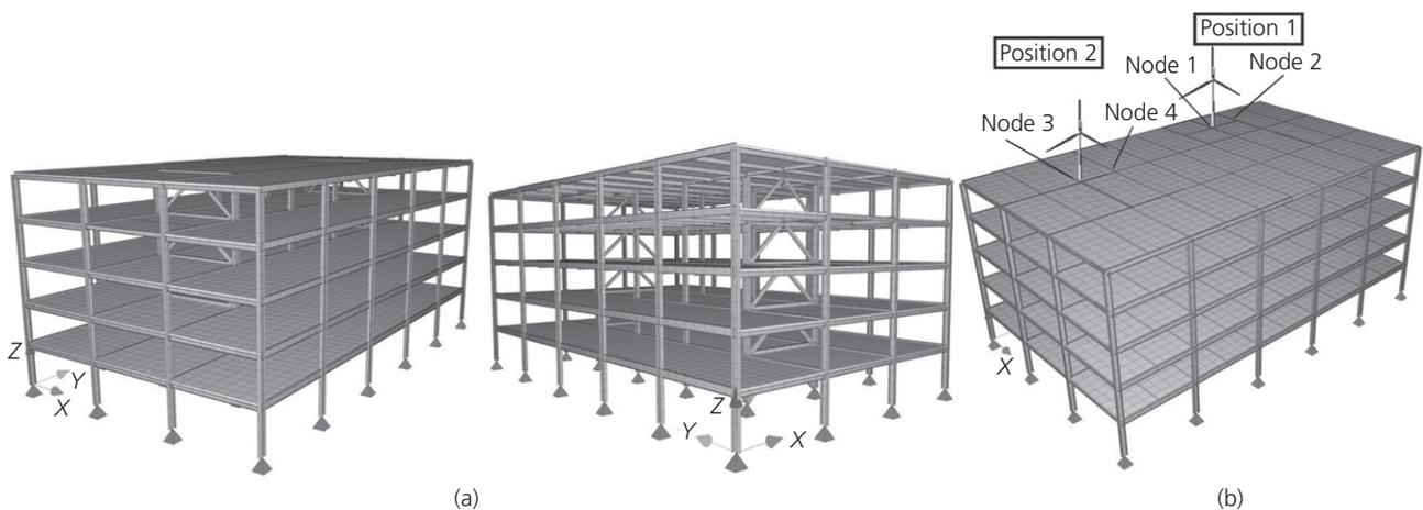
Figure 4. Numerical model of analysed steel building developed in Sofistik FE software: (a) steel building layout; (b) position of wind turbines
