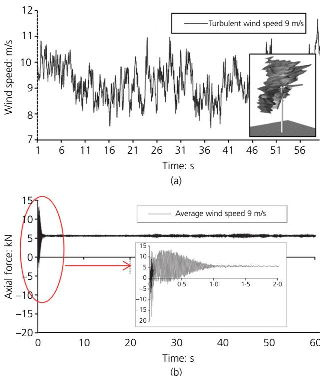
Figure 2. Development of SSWT in Ashes software package: (a) turbulent wind time-history generated by Ashes for 9 m/s average wind speed; (b) time-history of axial forces from wind turbine
