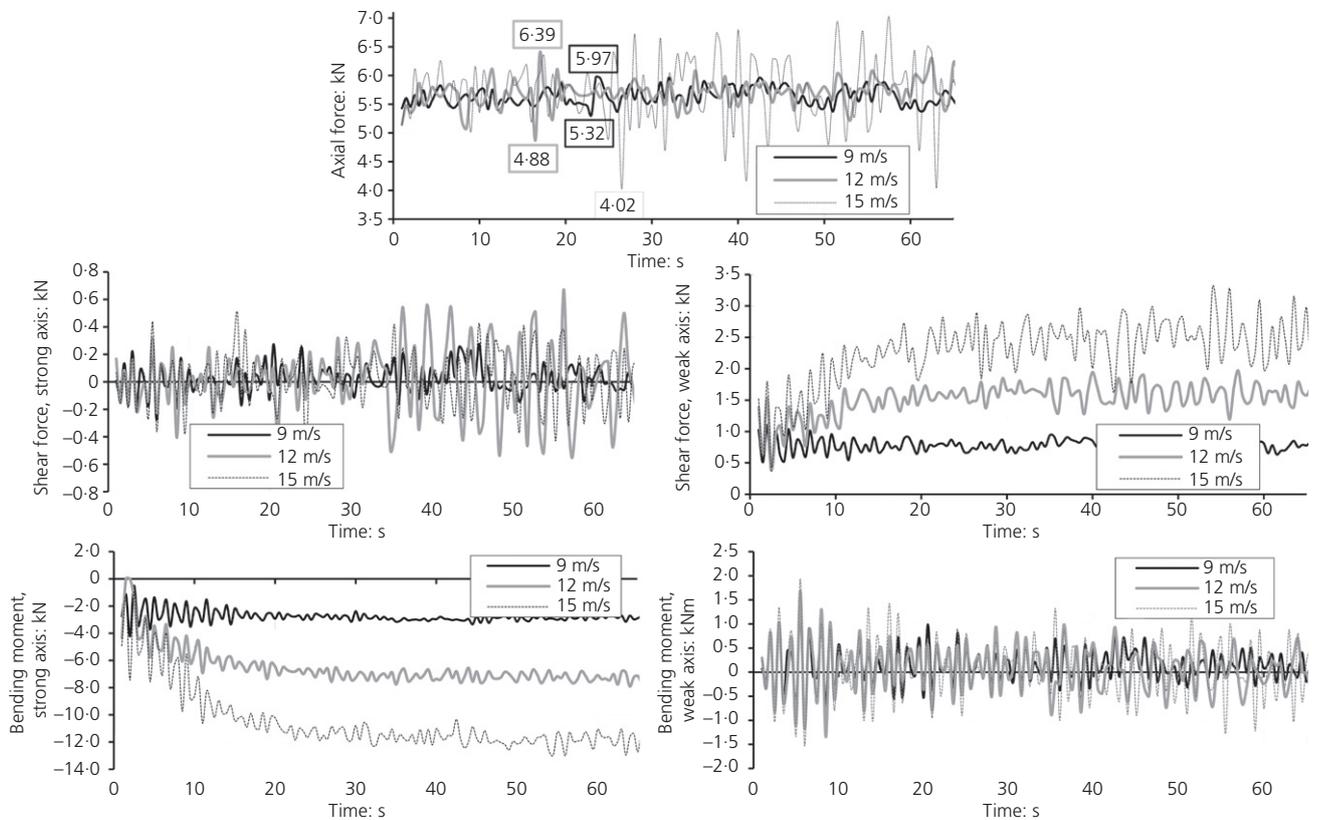
Figure 3. Time-history of forces and bending moments applied on the building's roof for average wind speeds of 9, 12 and 15 m/s
