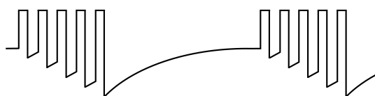
Figure 1.3: Burst spinal cord stimulation waveform
