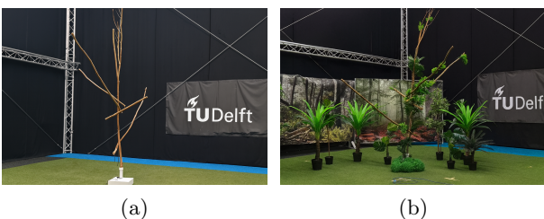
Figure 7: Controlled testing environment with the constructed 'tree'. The branches are easy to swap and adjustable for different angles. For CNN training and initial flight testing, the leafless tree was used (a). Green artificial foliage and forest scene banners are added in the background to add complexity on the right image (b).
