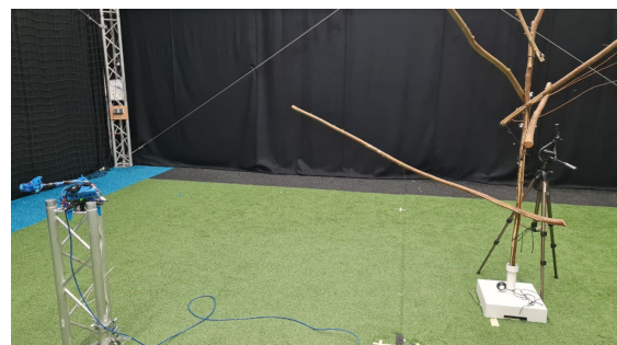
Figure 8: Static testing configuration with the drone mounted on a pedestal in front of branches at varying distances. Used to validate detection and transformation accuracy.
