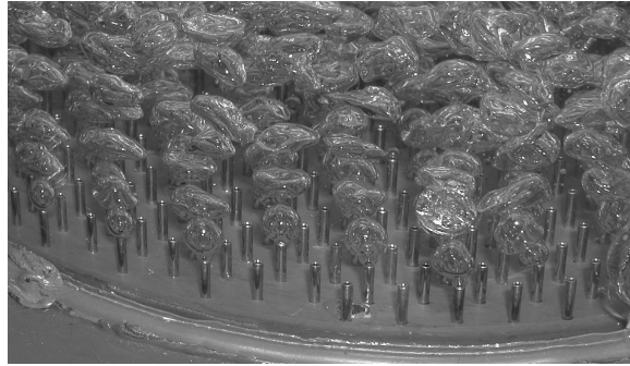
Figure 2.4.: Picture showing bubble formation with one third of the needles in operation.
