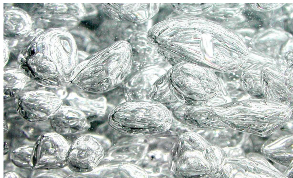
Figure 4.9.: Bubble shapes close to the wall in the cylindrical bubble column.
