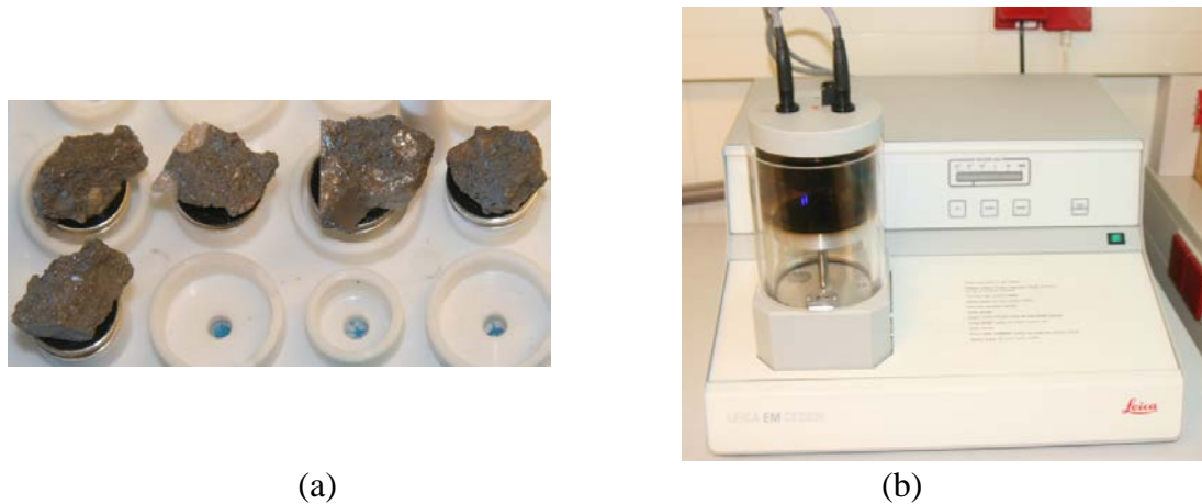
Figure 7.4: Carbon-coated samples for SE image observations (a) and carbon coating instrument (b)
