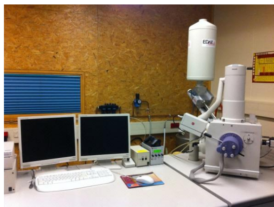
Figure 3.9: Philips-XL30-ESEM system for microstructural observation
