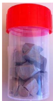
Figure 3.4: Cement paste blended with fly ash after stopping hydration and drying
