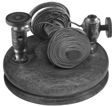
Figure 83: The first experimental electromagnet made in Albany by Joseph Henry (1829).
