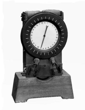
Figure 119: A model of the indicator of Wheatstone's ABC pointer telegraph (1840).
