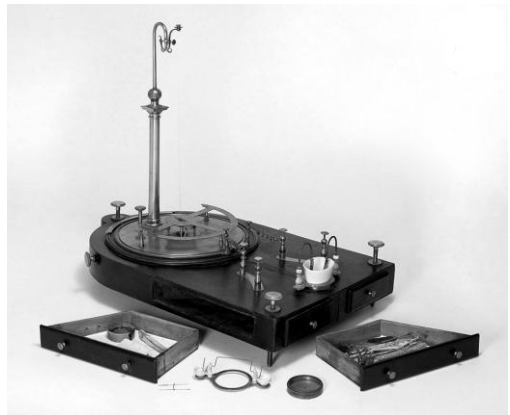
Figure 81: Nobili’s astatic galvanometer (1826).
