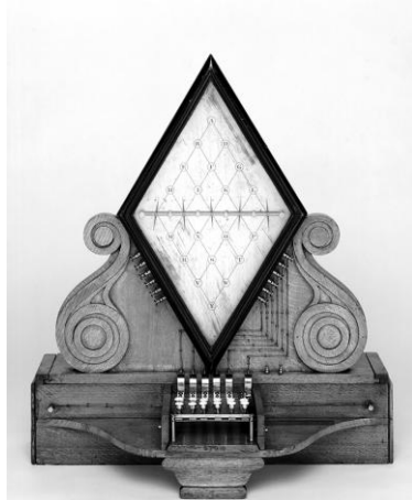
Figure 117: The final prototype of the Cook and Wheatstone five-needle Telegraph (1837).
