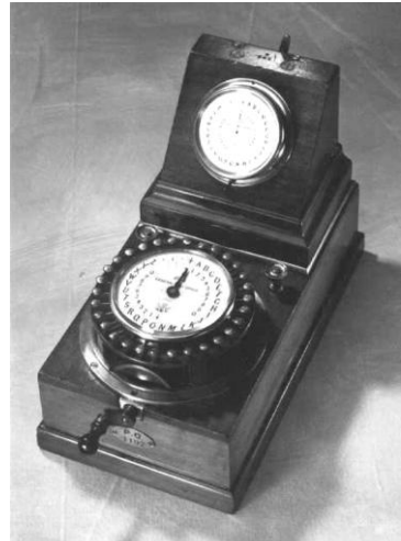
Figure 121: A later model of Wheatstone's ABC Pointer Telegraph (1858).
