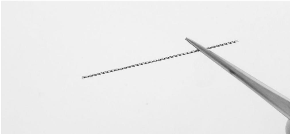
**Figure. 30** The as-manufactured porous SLM Ti6Al4V implant.
