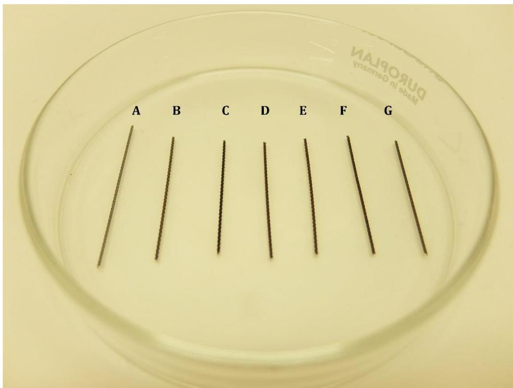
**Figure. 31** Porous SLM Ti6Al4V implants **A.** Before PEO processing and **B.** After PEO processing without NPs, **C-G.** with Ag NPs and pure Zn NPs.
