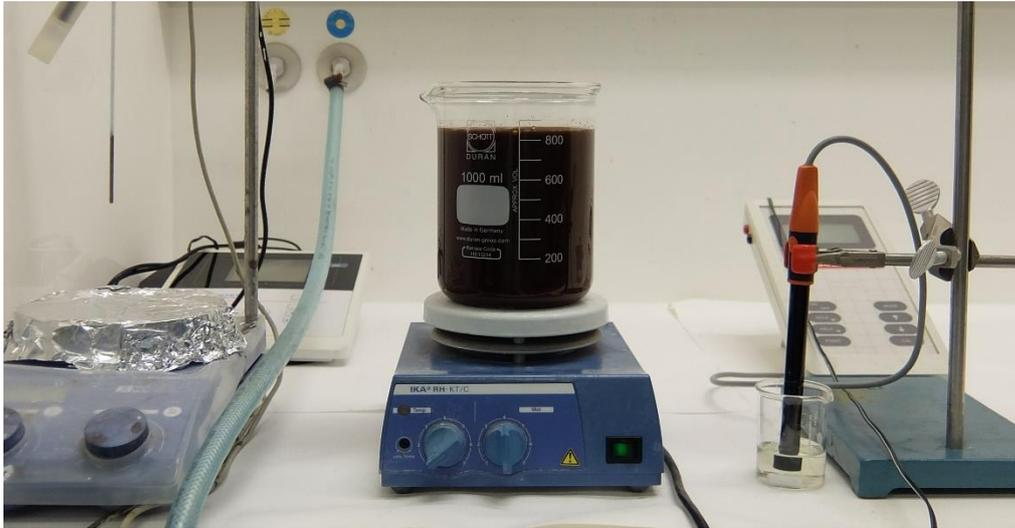
**Figure. 32** Calcium and phosphorus-based electrolyte for PEO processing with Ag NPs and pure Zn NPs.
