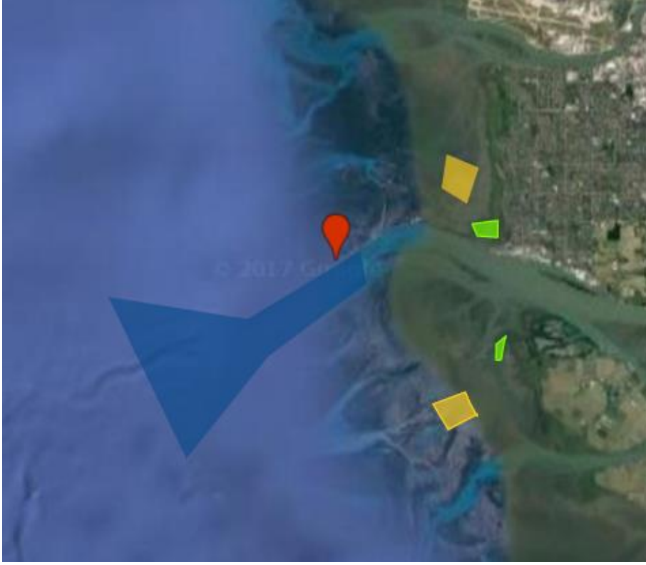
Figure 12 Training areas for spectral unmixing: blue is water, yellow is flat and green is marsh. The reference marsh fraction was found on the flat at the red marker.
