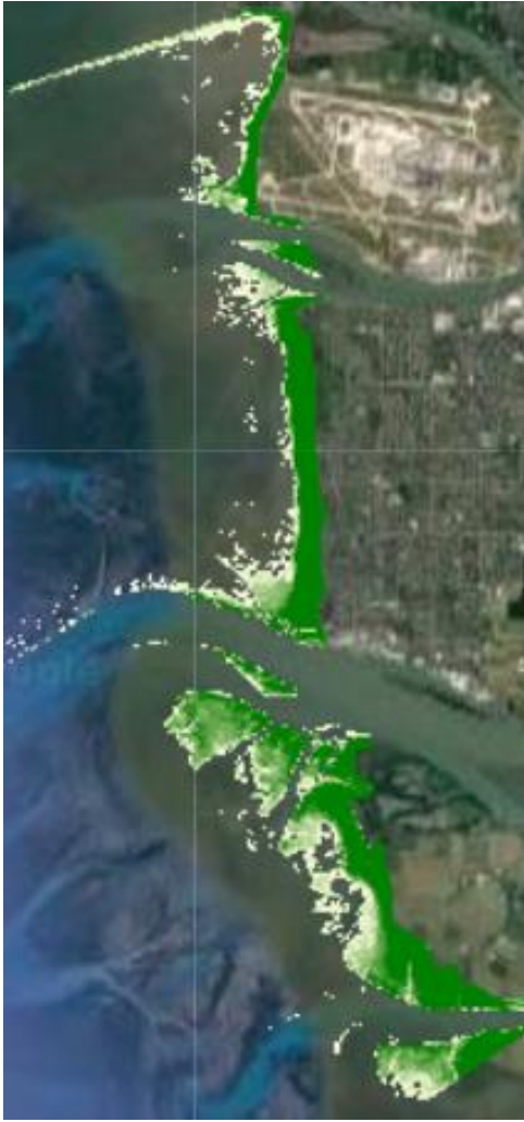
Figure 13 The result of the spectral unmixing procedure for marsh classification
