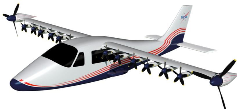
Figure 1.1: The NASA X-57 Maxwell conceptual aircraft with distributed propulsion and wingtip-mounted propellers [4].
