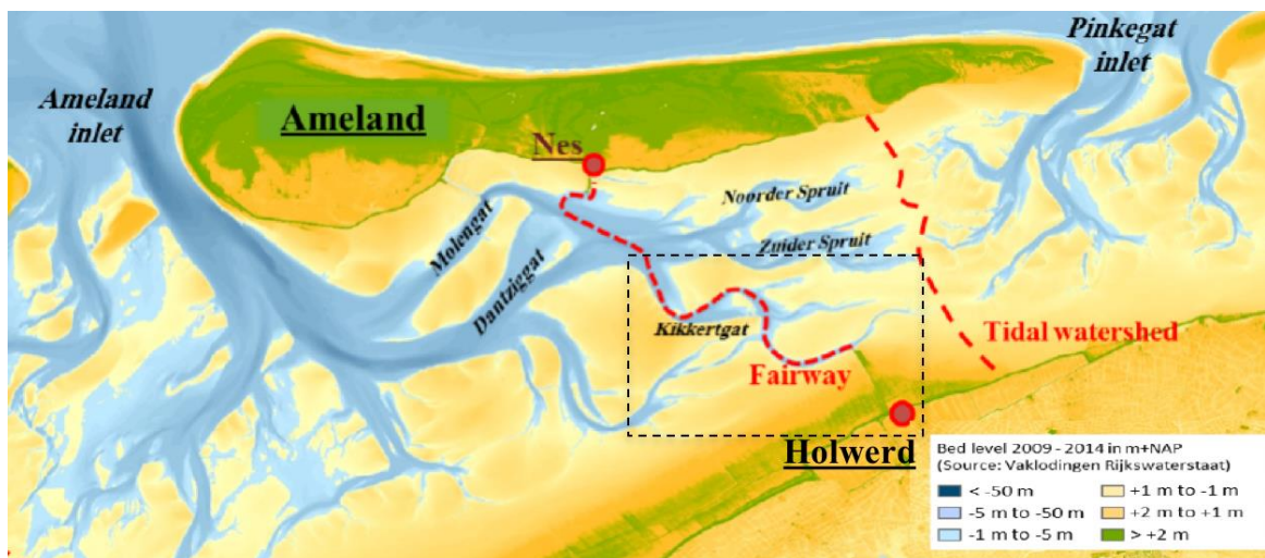
Figure 3-6: Bathymetry map of Ameland basin, location of the fairway and tidal watershed (van Til, 2017)
