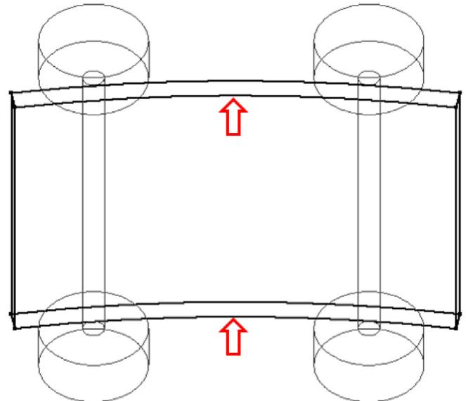
Fig. 5. Effect of lateral bending on a chassis [36].
