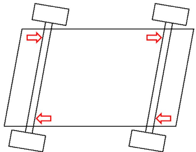
Fig. 6. Effect of horizontal lozenging on a chassis [36].
