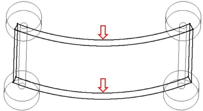
Fig. 4. Squatting effect due to acceleration [36].
