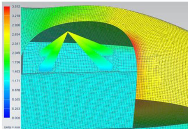
Fig. 10. Deflection result of chassis with enclosed doors.
