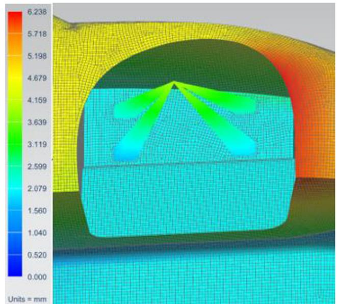
Fig. 12. Deflection result of chassis with compact doors.
