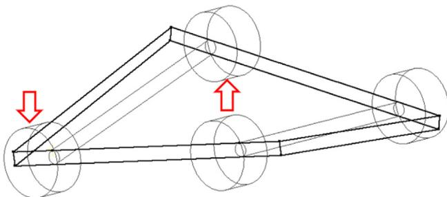
Fig. 3. Effect of torsional load on a chassis [36].
