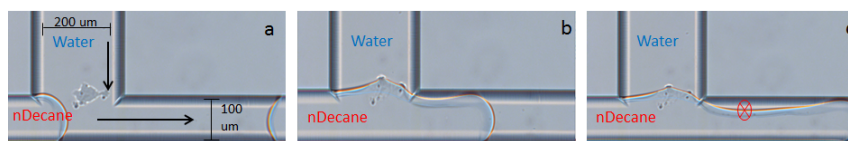
Figure 7.1: Reference case experiment for the T-Junction. Water and n-decane were co-injected at equal rates ( Q = 100 nl/min) to meet at the T-Junction. a-c show consecutive time steps.
