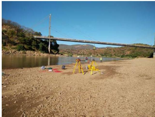
Figure 4.3 Set-up of a Differential GPS with a base- and rover receiver and an external antenna.
