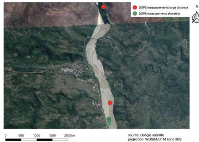
Figure 5.7 DGPS measurements of the water surface level for a short and large distance.
