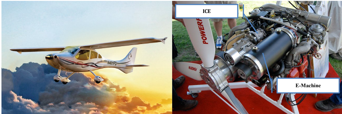
Figure 2-2: Flight Design C4 [53] (left) and parallel hybrid powerplant [54] (right)
