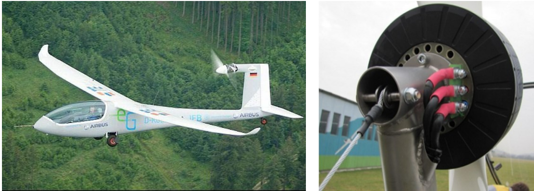
Figure 2-5: e-Genius aircraft [62] (left) and propeller with electrical motor [60] (right)
