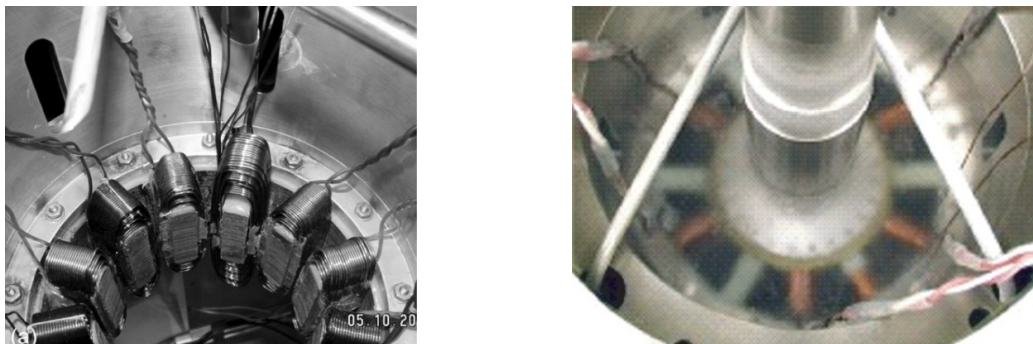
Figure 3-17: Cryogenic non-superconducting SRM stator [144] (left) with stator and rotor submerged in \text{LN}_2 [145] (right)
