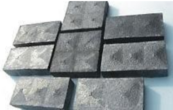
Figure 3-14: Samples of bulk material manufactured by THEVA [185]
