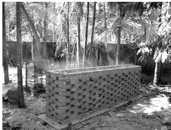
Figure 6.10 Plan, section (i) and picture (ii) of annular kiln enclosure for burning rice husk
