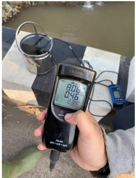
(c) Measuring the EC and pH with the Multimeter
