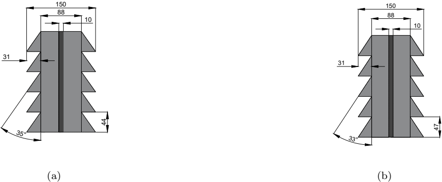
Figure 13: Schematic drawing of the design for prototype of Fin Design with measurements (a) 2D-design (b) Design for a slope of 20 degrees
