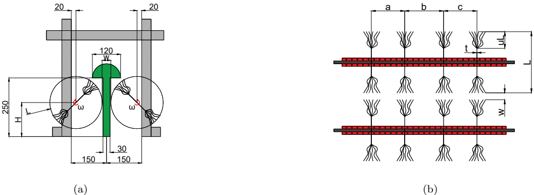
Figure 39: Schematic drawing of the Metal Wire design with letters given for the variables (a) Front view prototype (b) Top view shafts
