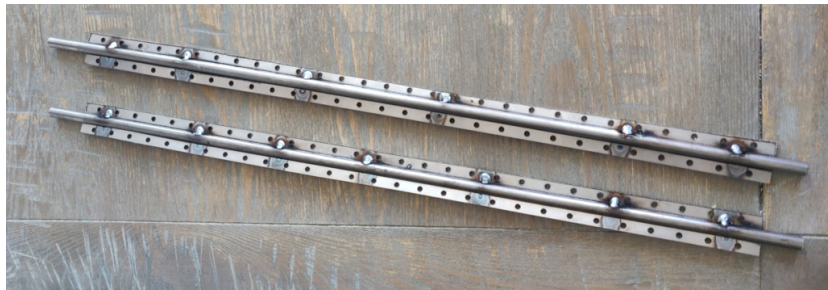
Figure 5: Steel shaft with a diameter of 10 mm with rectangular plates welded to the sides, containing holes every 20 mm
