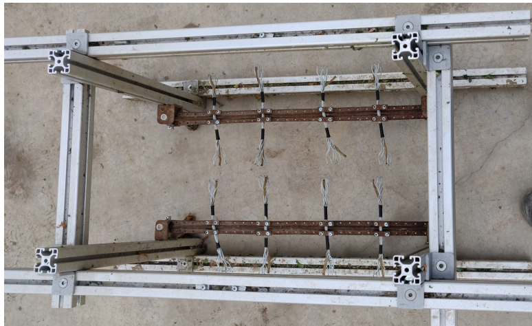
Figure 22: Example of the Metal Wire, with a 6 mm wire with unraveled ends
