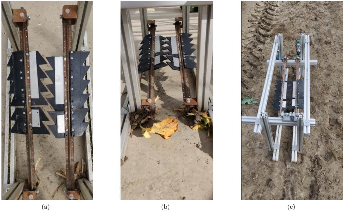
Figure 16: Pictures of the main frame with the Fin Design mechanism attached to the shafts (a) Close together showing designated holes (b) Slope of 20 degrees shown (c) Whole system
