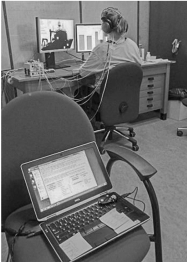
Fig. 4. Photograph of the experimental setup. In the foreground, a laptop shows the trainer part of COPE-FB system. In the background a participant views the ship simulation on the left display and the trainee part of COPE-FB system on the right display.
